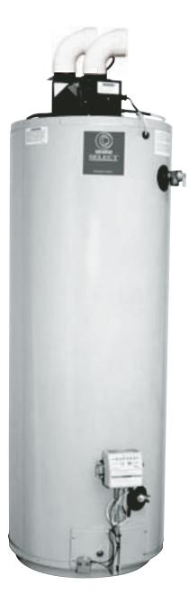
**Power Direct-Vent Design** – Two-pipe closed-combustion system draws all make-up air from outside the home, eliminating problems caused by insufficient indoor ventilation. For installation versatility, system permits combined horizontal and vertical venting and air intake runs up to 45 feet (including one 90° elblow using 3" Schedule 40 PVC, CPVC or ABS pipe.
